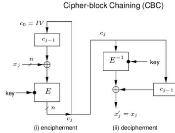
Figure 2: CBC Operation Mode of block ciphers
